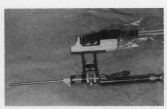
**Figure 4** Electromagnetic sensor attached to the Xomed XPS Straightshot débrider for intraoperative tracking.
