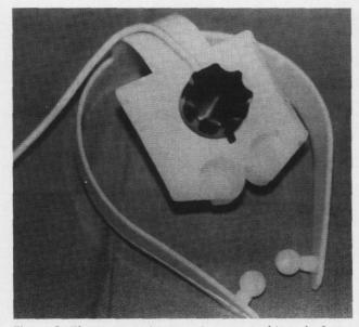
Figure 3 Electromagnetic sensor incorporated into the Instatrak headset.
